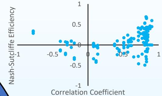
**Figure 5.** Nash-Sutcliffe efficiency, a measure of model accuracy, plotted against a correlation coefficient relating storm depth and time.
