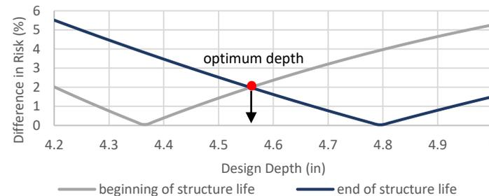
**Figure 4.** Graphical method for determining design depth. Percent deviation from the acceptable risk level is plotted for a range of depths.
